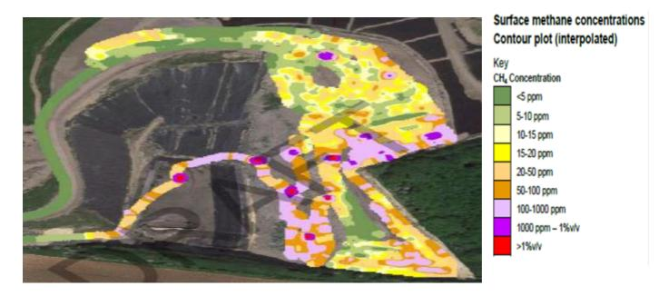
The diagram is the surface emissions concentrations contour plot. It shows that elevated levels of methane emissions are being released, especially around the leachate infrastructure. These can be easily identified as they are show up red on the contour plot.
